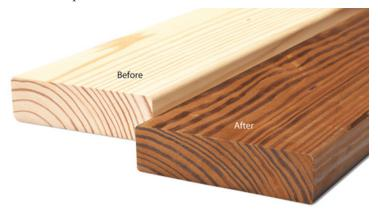
Figure 3: Thermal modification improves several characteristics of wood and imparts an attractive dark color to wood (www.popularwoodworking.com/projects/thermally-modified-wood)
