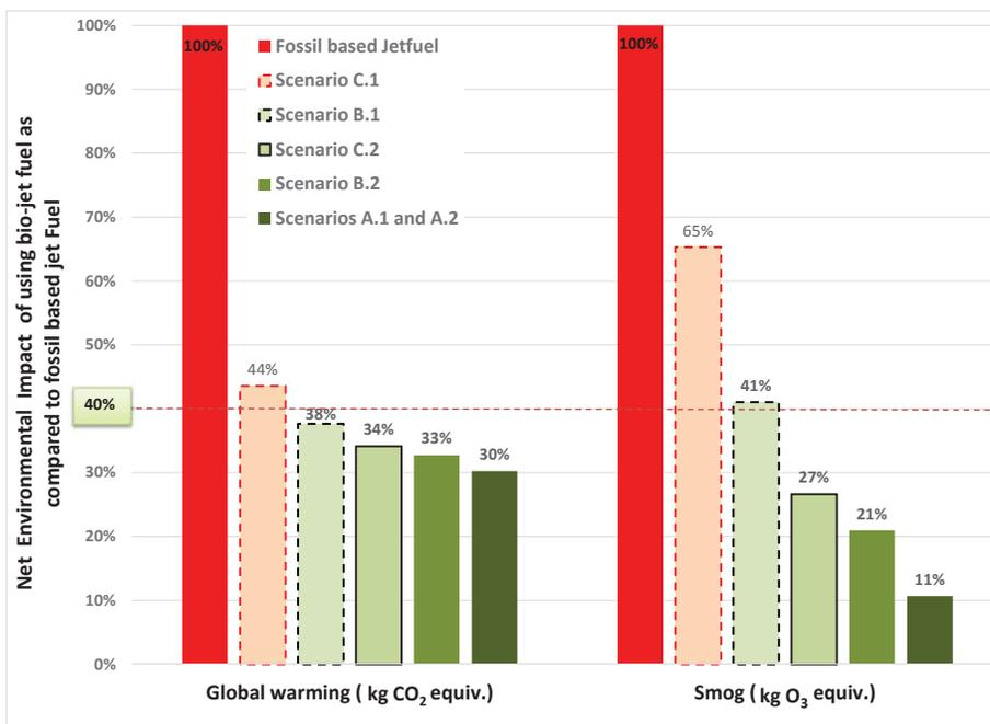
Figure 6. Net reductions in global warming and smog potential associated with bio-jet fuel used as a substitute for fossil-based jet fuel
