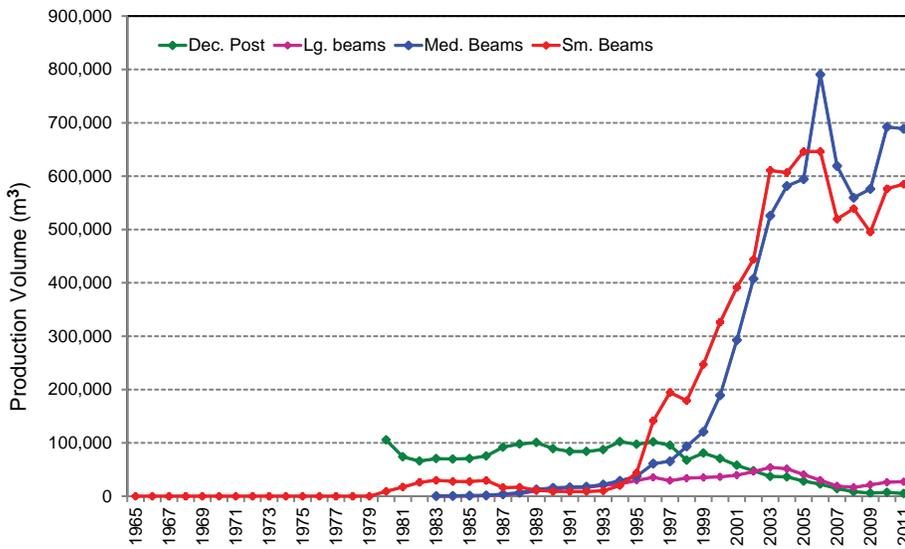
Figure 8. Japanese production of structural glulam lumber, by product.
