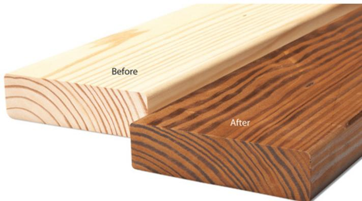
**Figure 3: Thermal modification improves several characteristics of wood and imparts an attractive dark color to wood**
