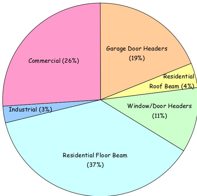
**Figure 2. Almost 70% of glulam beams are used in residential construction. (Source: APA 2007)**
